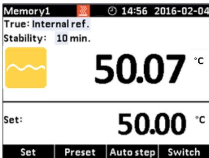
The calibrator has a set of internal stability criteria it shall meet before stability is indicated. The stability time may be set beyond the internal stability criteria. The stability time can be set (in minutes) using integers from 5 – 99
