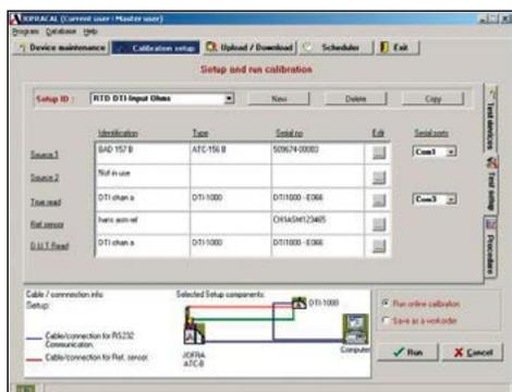
JofraCal is a highly versatile calibration software that is supplied together with the PTC calibrators. The software ensures easy calibration of all kinds of temperature sensors, such as RTD's, thermocouples, transmitters, and thermoswitches. Furthermore, it can be used for pressure calibration i.e. pressure gauges and pressure switches. JofraCal integrates with Jofra calibration instruments. As for temperature calibrators, it is the whole range of temperature
