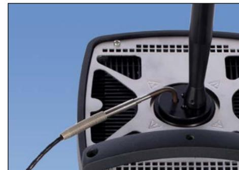
The STS-150 reference sensor is specially designed with an angled 90° rod, and customized to fit the calibrator so that it is only slightly higher than the top of the PTC calibrator. The unique design makes it possible to calibrate threaded sensors and sensors with connection heads without any problems. The STS-150 reference sensor also alerts you when your calibration has expired.
