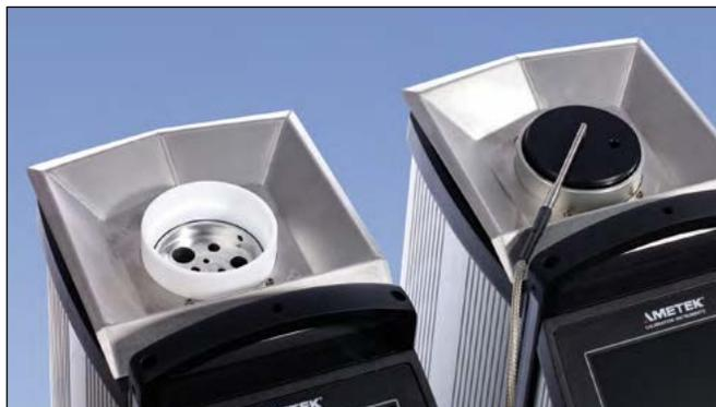
The RTC-158/250 calibrators are fitted with a 160 mm (6.3") deep well with a diameter of 63.5 mm (2.5"), which are twice the size of any other dry-block. And, they can be used both as dry-block calibrators and as liquid calibration baths with a magnetic stirrer.
