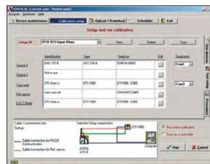
JofraCal is a highly versatile calibration software that is supplied together with the RTC calibrators. The software ensures easy calibration of all kinds of temperature sensors, such as RTD’s, thermocouples, transmitters, and thermoswitches. Furthermore, it can be used for pressure calibration i.e. pressure gauges and pressure switches. JofraCal integrates with Jofra
