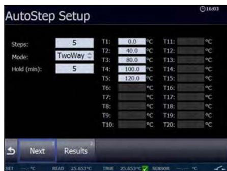
Up to 20 different temperature steps may be programmed including the hold time for each step. Upon completion of an auto-step routine, the user can easily read the results for the sensor-under-test on the RTC display. Results from twenty auto-step calibrations are stored.
