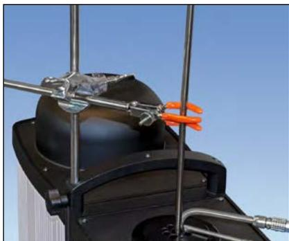
The integrated support rod is part of the reduced weight philosophy. It is lightweight and very easy to mount on the RTC. Two fixing holes are integrated in the calibrator where the support rods can be mounted.
