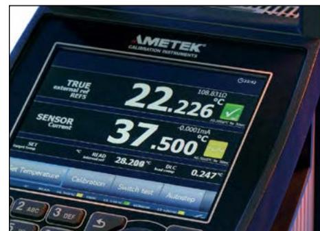
The navigation is menu-driven and very logical to use, and the display shows any important information needed for the current function in use. The communication windows pop up and are followed by discrete sound messages. The display is very bright, and the main information can easily be read from a distance. The advanced simplicity RTC user interface is available in English, German, Chinese, and Japanese.
