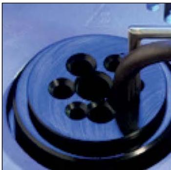
Two special multi-hole insert kits have been developed to comply with the calibration of almost any sensor diameter without having to buy numerous inserts.
