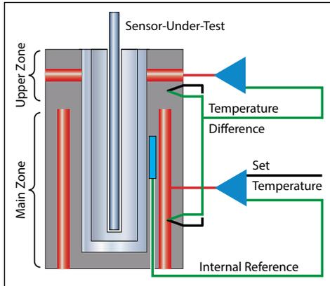
The RTC series of calibrators provide precision temperature calibration of sensors, whatever the type or format. This is accomplished through an innovative active dual-zone heating technology.
