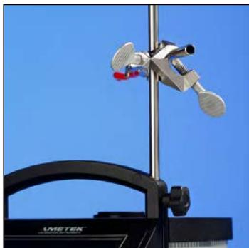
The new integrated support rod is part of the reduced weight philosophy. It is lightweight and very easy to mount on the RTC. Two fixing holes are integrated in the calibrator where the support rods can be mounted.
