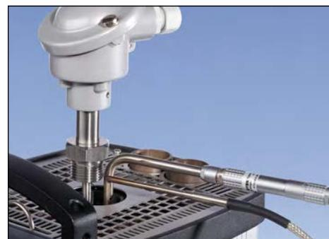
The STS-200 reference sensors and the DLC sensors have been specially designed. They are both angled 90° and have been customized to fit the calibrator so that they are only slightly higher than the top of the RTC calibrator.
