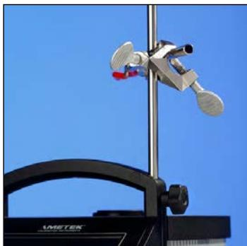
The integrated support rod is part of the reduced weight philosophy. It is lightweight and very easy to mount on the RTC. Two fixing holes are integrated in the calibrator where the support rods can be mounted. And even though its weight has been reduced by 50%, the support rod will remain very firmly positioned.
