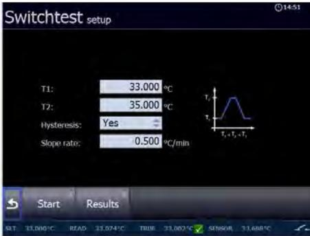
If no change in the switch position is registered during the test a red cross will be displayed in the Result list instead of a green check ✓.
