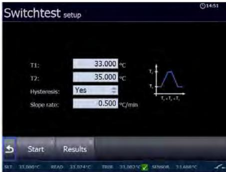
A Switch test setup menu is displayed.
