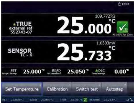
The functions in the horizontal menu are available using the soft keys or the arrow keys on the keyboard (see description in section 4.3).
