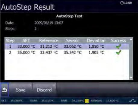
The screenshot shows the 'AutoStep Result' screen. At the top, it says 'AutoStep Result' and 'AutoStep Test'. Below that, it displays 'Date: 2009/06/19 13:07' and 'Steps: 2'. A table shows the results for two steps:
