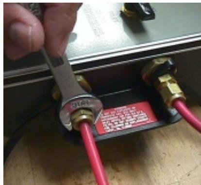
*Connect instrument to be tested to the OUTLET valve.*
