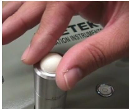
*Carefully, lift the ceramic ball from the nozzle assembly and store in a secure location.*
